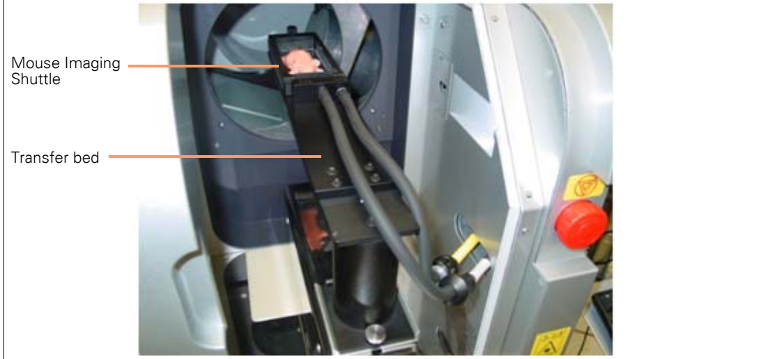
Figure 7.2 Quantum FX \mu CT Scanner with Mounted Transfer Bed and Mouse Imaging Shuttle
