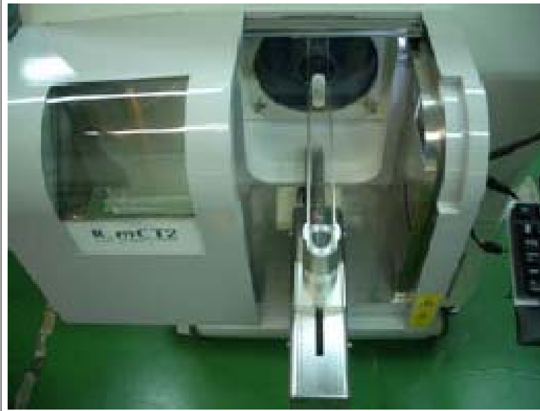
Figure 6.6 Sample Bed at the Out-Limit Position
