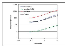
*Figure 7.* LANCE instrument performance for peptide dilution series measured with black OptiPlate-384.
