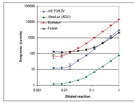
*Figure 8.* LANCE instrument performance for diluted reaction measured with black OptiPlate-384. X-axis presents the dilution factor where 1 is composed of 10 nM peptide, 50 nM SA-APC and 1 nM Eu-labled anti-P-Tyr antibody diluted in the assay buffer and where 0.1 corresponds components diluted 1:10 in the reaction buffer.
