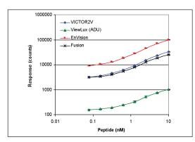
Figure 5. LANCE instrument performance for peptide dilution series measured with white OptiPlate-384.
