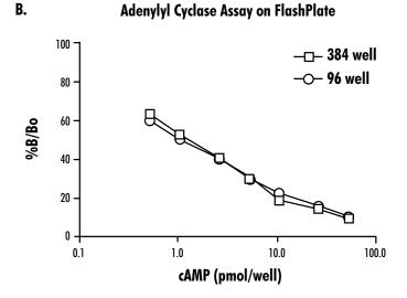
Cyclic AMP standard curves were run in an Adenylyl Cyclase assay on both 96-well and 384-well antibody-coated FlashPlates. As shown in Figure 1a, the assay signal on the 384-well plate was approximately one-half that of the 96-well plate. However, Figure 1b shows that when the assays are both normalized by %B/Bo, performance is the same. The signal observed in the 384-well version of the assay was still high enough to be considered robust.
