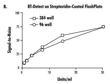
A Reverse Transcriptase assay was run on both 96-well and 384-well streptavidin-coated FlashPlates. Figure 2a shows that assay signal from the 384-well plate was approximately half that of the 96-well plate. But as shown in Figure 2b, the signal-to-noise ratio was unchanged.
