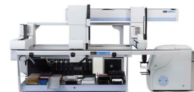
The JANUS MDT™ Automated Workstation with a 384-tip modular arm was used to dispense reagents to the low-volume 384 and 1536-well plates. The Envision MultiLabel Reader was used to read all assay plates.
