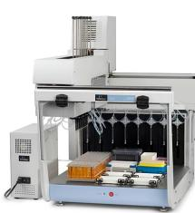
The Varispan arm employs positive displacement pipetting, with variable tip spacing that allows for reformatting of samples, such as transfer from test tubes or microfuge tubes to microplates, and "cherry-picking". Also, with the Versatip option, the user can elect to use fixed tips or disposable tips, and switch modes within a test.
